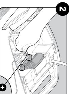
Using a short screwdriver open the 2 screws.
